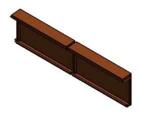
HAT TRACK STYLE FASCIA PANEL SYSTEM WITH FASTERNERS ON TOP OF PARAPET AND BOTTOM OF FASCIA.
